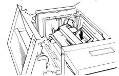
**6** Close the printer cover. Push down on the cover to lock it into position.
